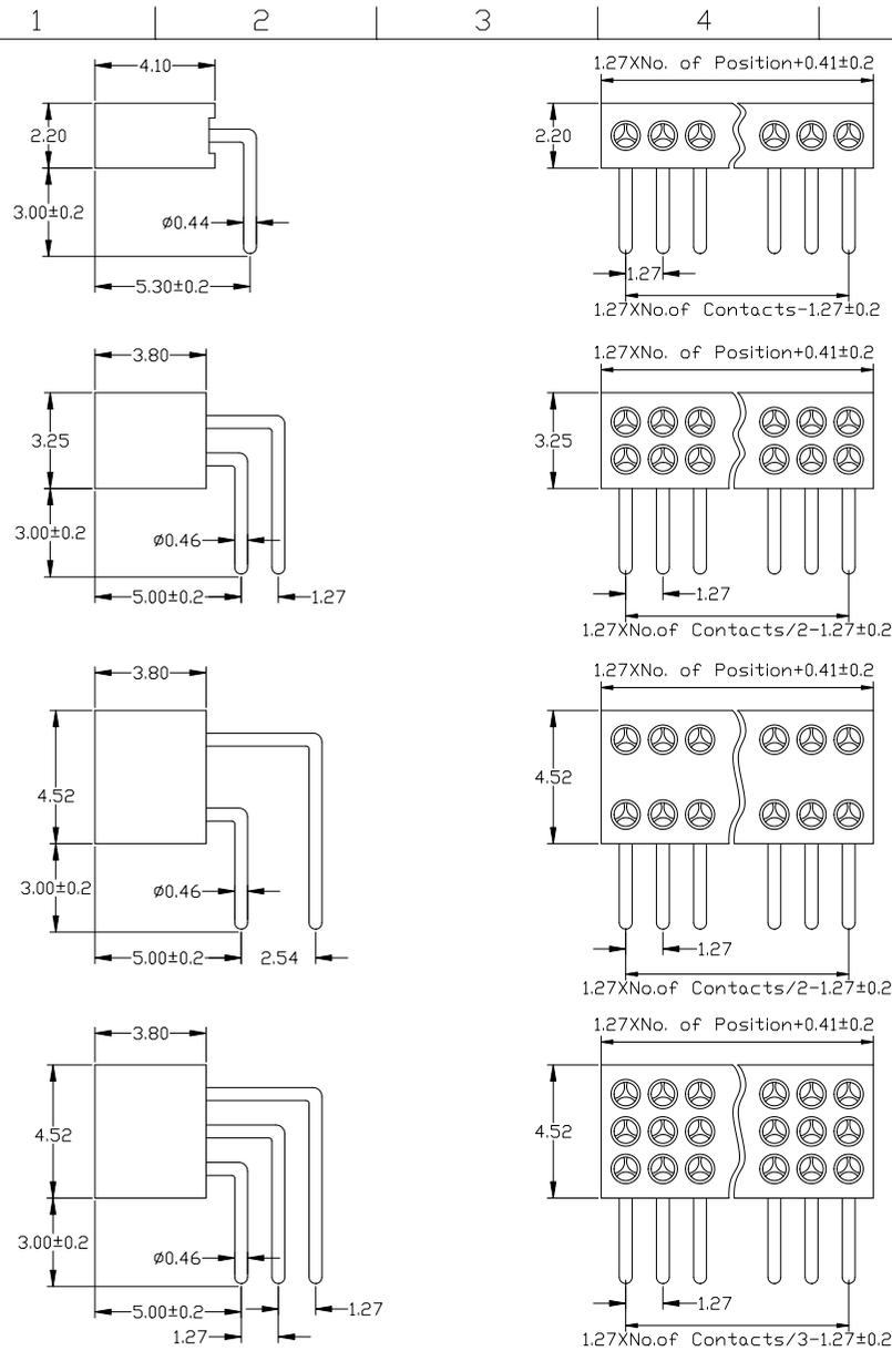
Right socket connector:solder tail
